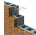
Block Reinforcement (Ladder Type & Truss Type)
